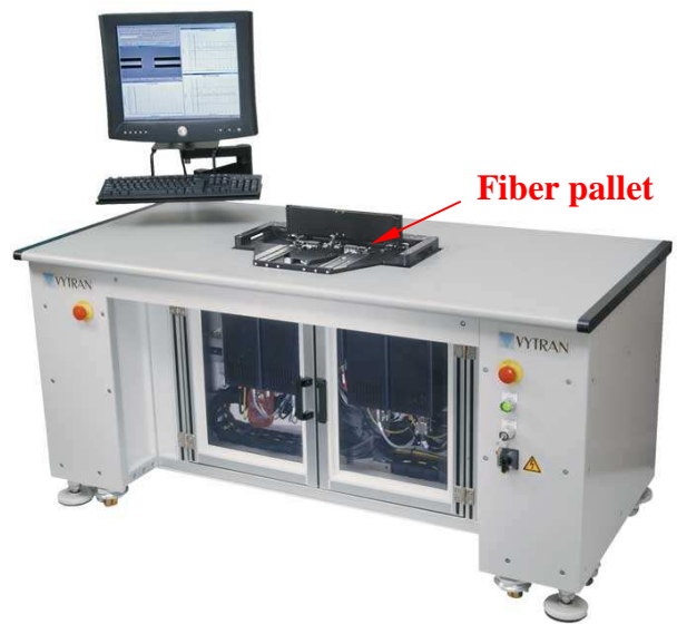
Fig. 16 An automated splicing system example
